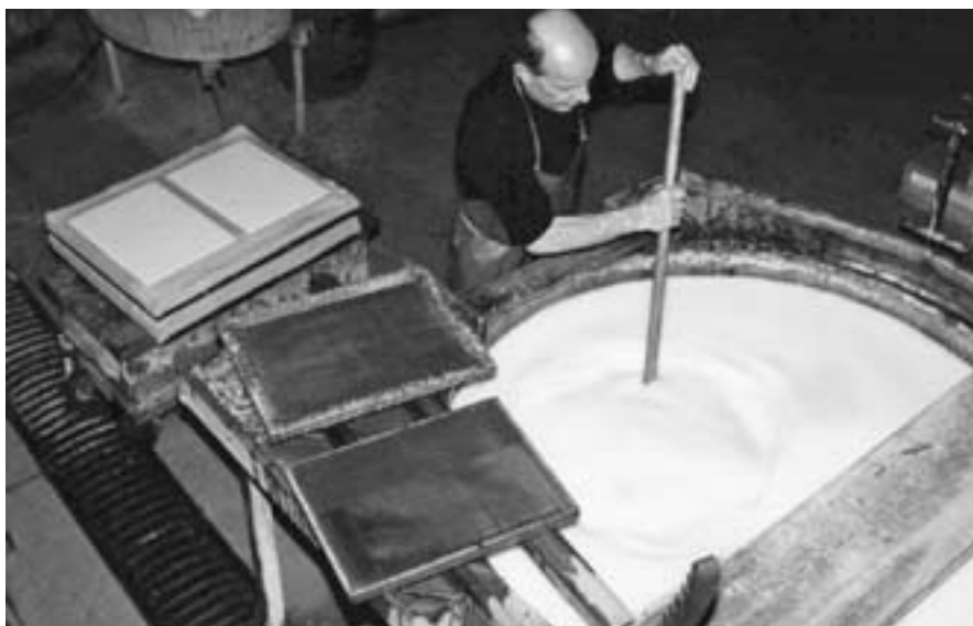
Bill Walker, foreman of the beater room, has Pakehas as well as Maoris working for him. The chemicals and other constituents are mixed together. The mixture determines the quality of the board.
